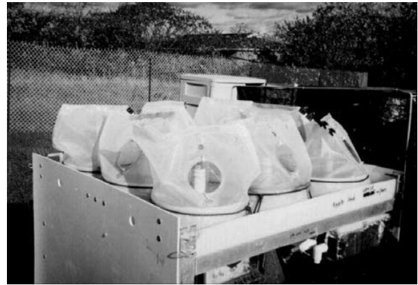
Fig. 1 A modular mesocosm table containing eight replicate artificial streams each covered in emergence traps.
