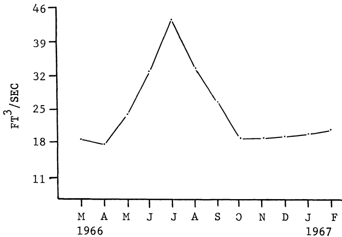
FIG. 4. Daily mean flow of coolant water leaving Boomer Lake power plant.
