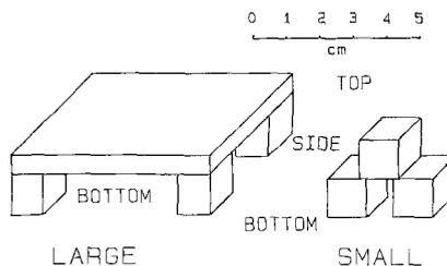
**Fig. 1.** Configurations of the small and large artificial substrates used in the experimental streams noting the upper (i.e., top and side) substrate surfaces. A single layer of glass beads (4 mm diameter) filled the interstitial spaces between and beneath the substrates
