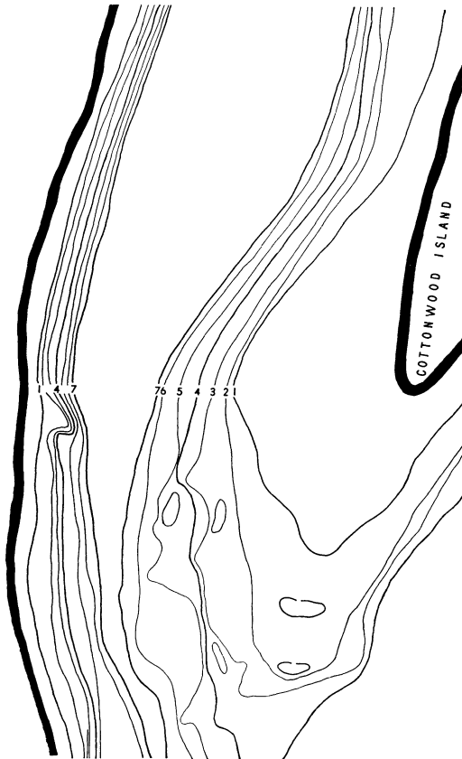
FIG. 5. Topographic detail of lower end of Cottonwood Chute, showing constriction of the channel at lower depths.
