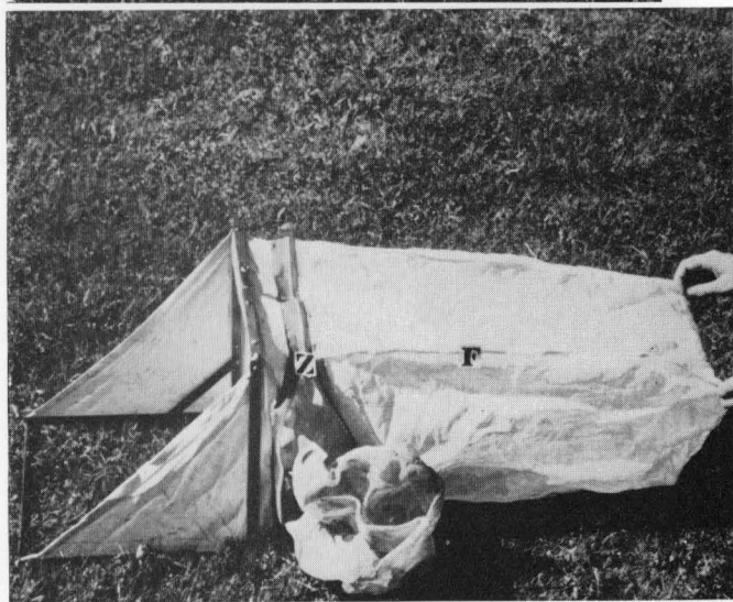
Plate 1. Upper: double-bag dip-net sampler; lower: double-bag Surber sampler. C, coarse mesh; F, fine mesh; Z, zipper.
